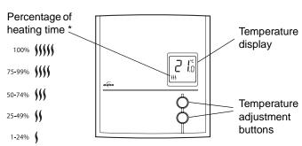
\* The thermostat displays the percentage of heating time required to maintain the desired temperature. For example, §§ is displayed when heating is activated 40 percent of the time.
